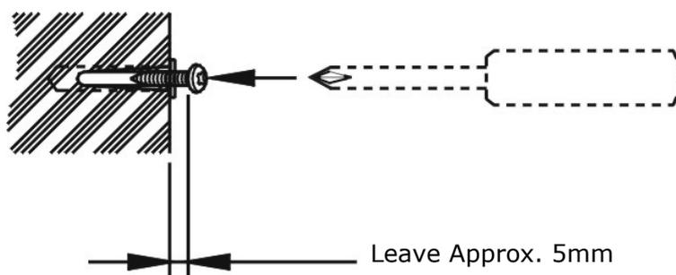
5. Mount the antenna on to the wall.
