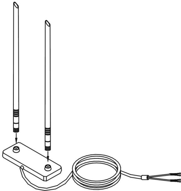
2. Attach the antennas to ZSR9104WE by connecting 2 antenna connectors at the end of the cable.
