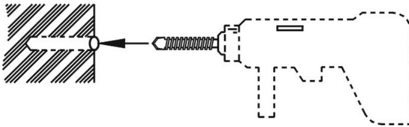
**Note:** Ensure you are using the 3mm (1.8 inch) drill bit size and type for the wall.
