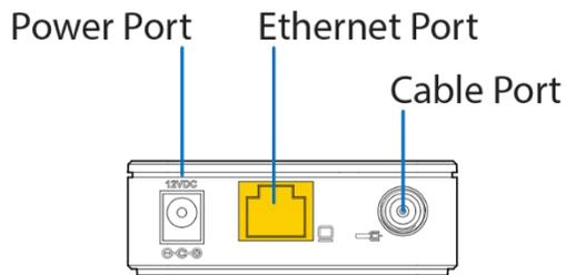
**Power Port**—Connect the included AC power adapter to this port.
