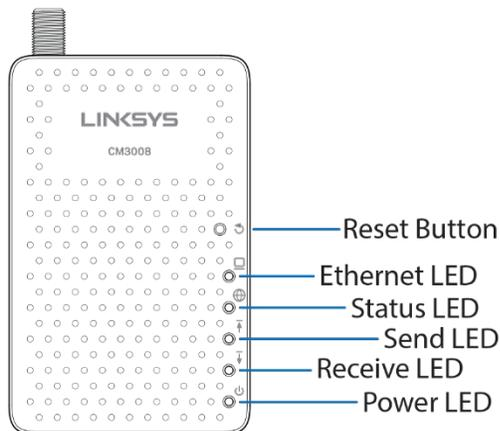
**Reset Button**—Press and hold for five seconds to restore settings to factory defaults and reboot the modem.
