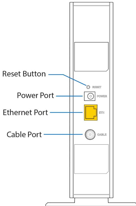
**Reset Button**—Press and hold for five seconds to restore settings to factory defaults and reboot the modem.
