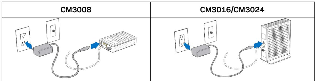
**Note**—If your modem is equipped with a power switch (located on the back panel), make sure that the switch is in the ON position to provide power to the modem.
