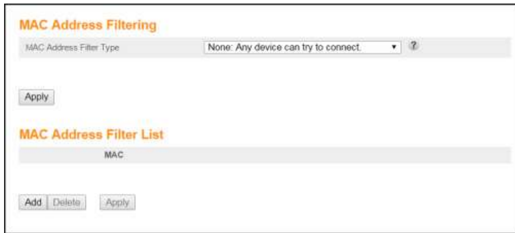
Figure 35: Set Up MAC Filters Screen
