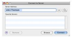
In the **Server Address** box, type **smb://<server name>**, where <server name> is the Server Name you assigned to your USB storage device (default: **smb://THOMSON**).
