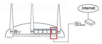
2. Connect all your computers and network devices (network-enabled consumer devices other than computers, like game console, or switch / hub) to the LAN port of the router.
