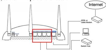
3. Connect the A/C power adapter to the wall socket, and then connect it to the 'Power' socket of the router.
