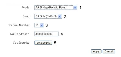
NOTE: Two wireless routers must use the same mode, band, channel number, and security setting!
