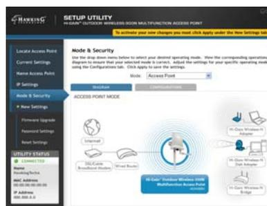
The included Windows based Setup Utility is a powerful tool for administrators to configure and troubleshoot settings on the HOWABN1. The Setup Utility allows administrators to upgrade firmware, reset devices to factory settings, adjust IP settings, change operating modes and view current system
