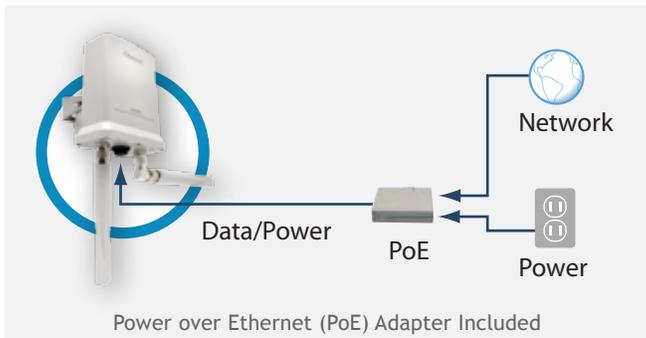
By combining your power and data connections into a single cable, PoE simplifies the setup of the Hi-Gain Outdoor Multifunction Access Point. The included Power over Ethernet DC Injector provides power and network access (through your home or business router or network connection) and combines them into a single RJ-45 connection for the HOWABN1. This allows you to install the HOWABN1 outdoor in hard to reach locations without worrying about running both power and Ethernet cables.
