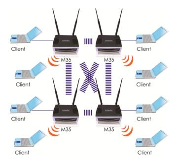
In Mesh Mode, recommended 1 Gateway with 4 Relay Linear and radiative deployment scenario.
