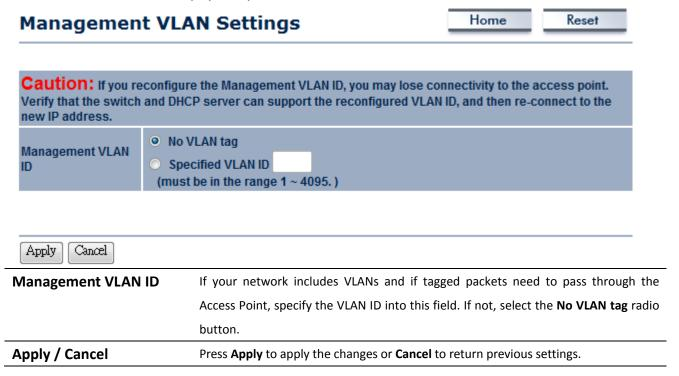
Auction: If you reconfigure the Management VLAN ID, you may lose connection to the M35. Verify DHCP server can support the reconfigured VLAN ID, and then re-connect to the new IP address.
