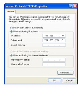
Auction: IP Address entered in the TCP/IP Properties needs to be at the same subnet of the M35 IP Address. For example: M35's default IP Address is **192.168.1.1** so the IP Address in the TCP/IP settings could be **192.168.1.10**.
