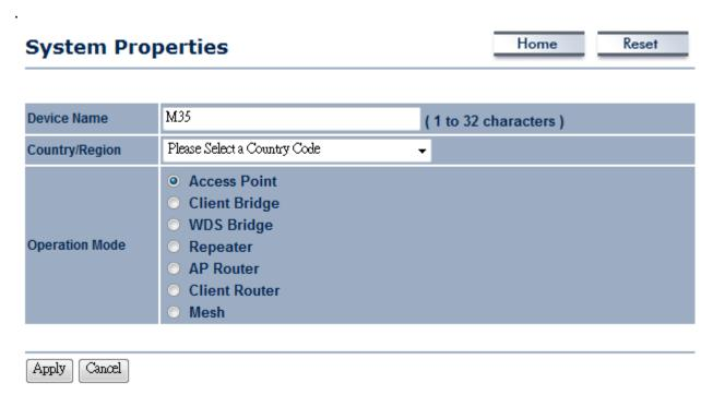
**Device Name**: Specify a name for the device, but it is not the broadcast SSID. It will be shown in SNMP management.
