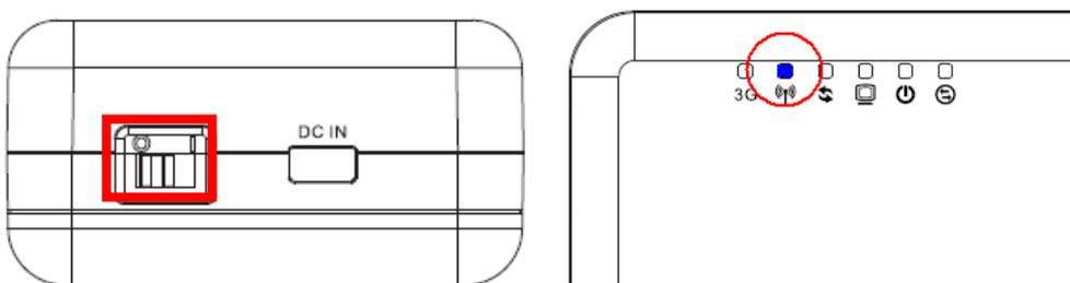
**Note1:** You are advised to flip on/off switch to **0+** before charging the battery. It takes about 1~2 hours to charge the battery.
