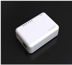
ETR9350 is a 2T2R Wireless Single chip 11N Pocket AP/Router that delivers up to 6x faster speeds than 802.11g devices so it can drive superior performance and unparalleled wireless range. With easy to use WPS function it helps users to have wireless connection quickly.
