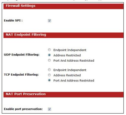
Enable SPI: Place a check in this box to enable SPI. SPI ("stateful packet inspection" also known as "dynamic packet filtering") helps to prevent cyber attacks by tracking more state per session. It validates that the traffic passing through that session conforms to the protocol. When the protocol is TCP, SPI checks that packet sequence numbers are within the valid range for the session, discarding those packets that do not have valid sequence numbers. Whether SPI is enabled or not,
