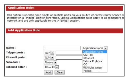
Name: Assign a meaningful name to the virtual server. Several well-known types of virtual server are available from the Application Name drop-down list. Selecting one of these entries fills some of the remaining parameters with standard values for that type of server.
