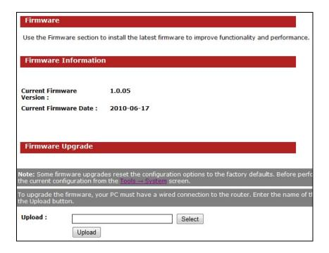
Ensure that you have downloaded the appropriate firmware from the Encore's website. Connect the EN2HWI-N3 Router to your computer using an Ethernet cable, as the firmware cannot be upgraded using the wireless interface.
