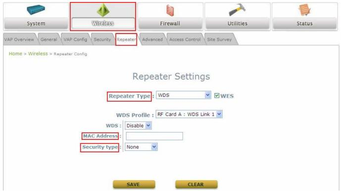
To extend its wireless coverage, EAP700 is capable of creating WDS links for connection to other WDS-capable APs (peer APs). EAP700 supports up to 4 WDS links; by default, all WDS profiles are disabled.
