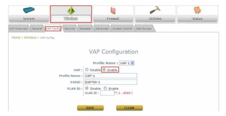
EAP700 Supports up to 8 virtual APs. By default, only 1 VAP is enabled.
